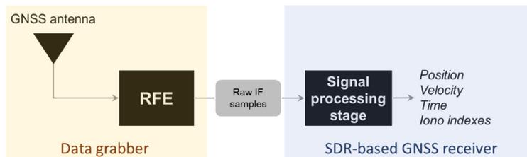
**Figure 1** The architecture of an SDR-based GNSS receiver.
