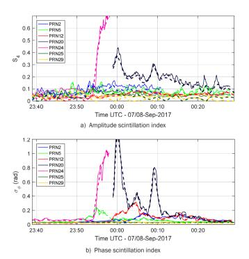
Figure 6 Comparison of scintillation indexes for GPS L1 C/A signals – Septentrio PolaRxS receiver (dashed line) vs. software receiver (continuous line).
