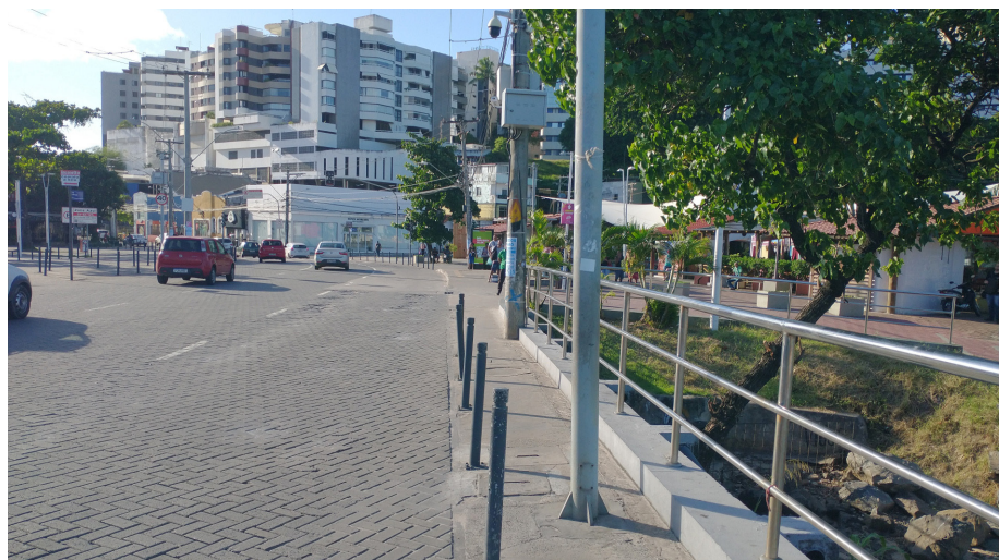
Figure 6: Shared traffic lane in Largo da Mariquita, where the pedestrian-only section has serious mobility issues caused by the installed poles. Source: Photograph by the author taken on June 11, 2024.
