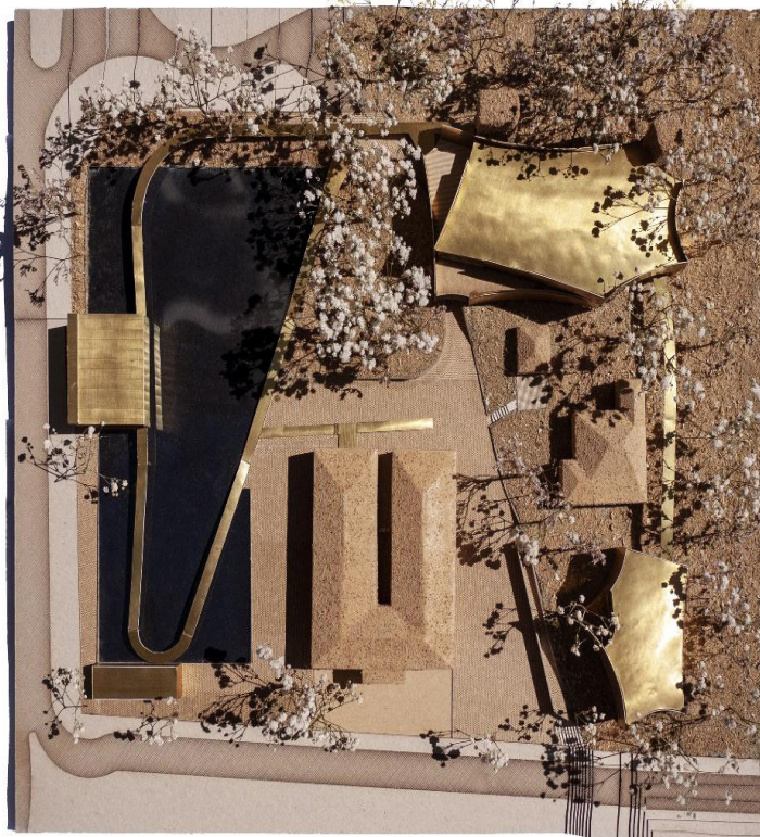
Figure 3: Physical model, the configuration of the version presented in the Competition. Reflected in black is the water mirror, proposed in correspondence with the underground reservoir chambers. In metal, the new buildings and walkways are represented, including the pipeline structure enclosure and the high-voltage cabin. The buildings adapted to the tree masses with an exhibition area, auditorium, and library. Source: SIAA.
