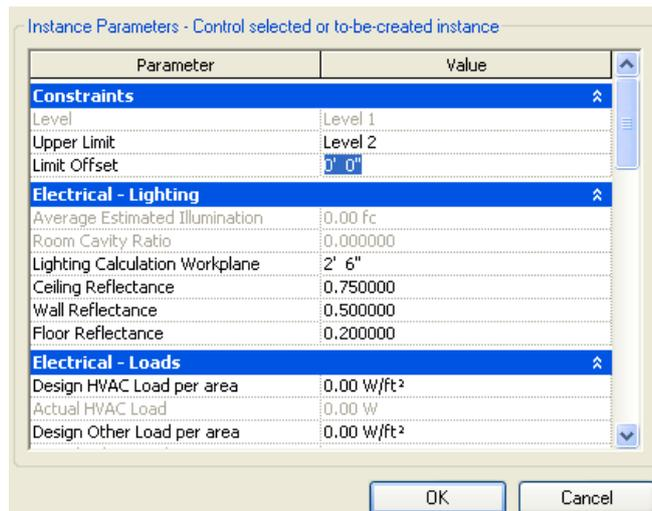
Figure 6: Settling the “Upper Limits” in a Revit model
