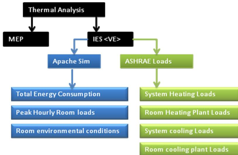
Figure 2: Thermal loads calculations in IES<VE>
