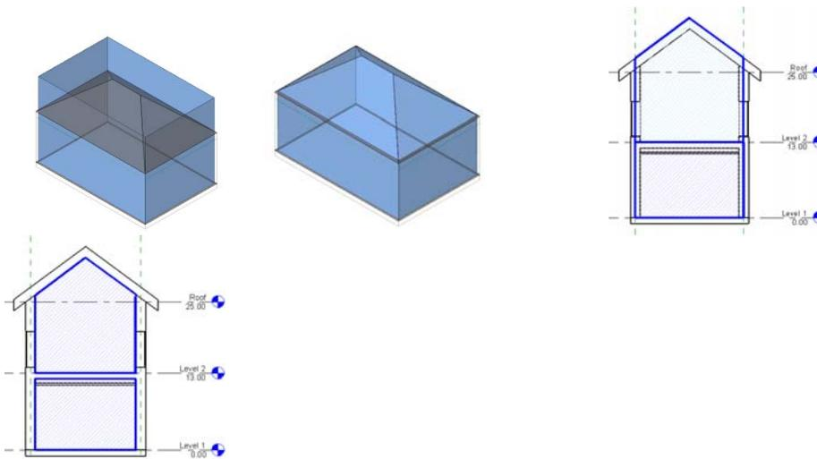
Figure 3: A model showing analytical volumes with the “Compute Room Volume” toggle off and on
