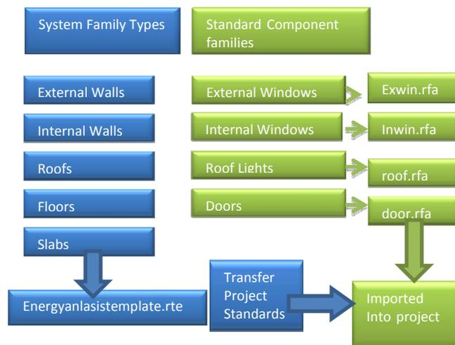
Figure 13: Development of the system family types and standard component families
