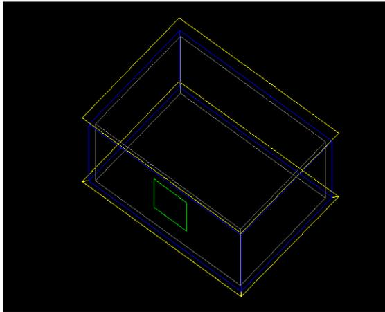
Figure 5: The blue line in IES shows analytical volume and grey shows inner volume
