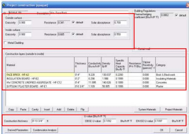
Figure 14: Project constructions for a 4 inch face brick wall type
